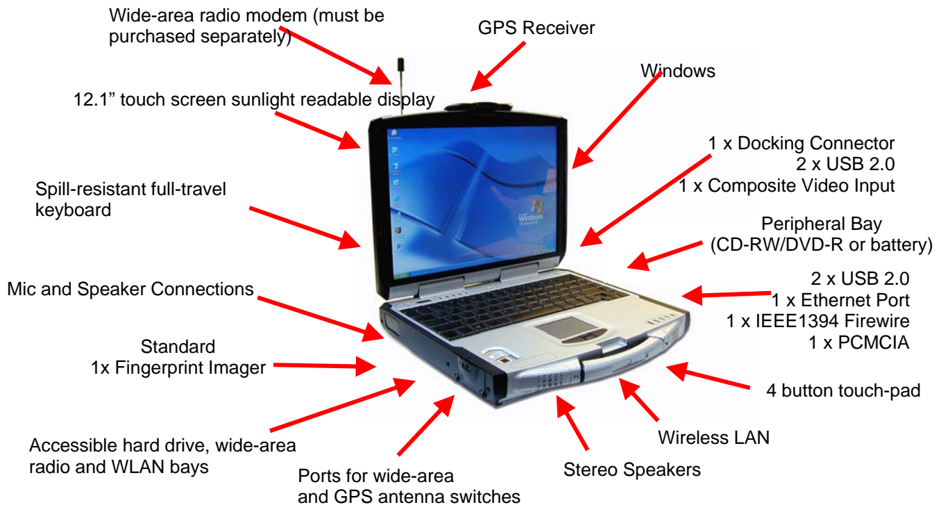
Figure 10-5 - The figure above shows some of the features of the ML900 laptop
